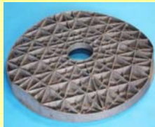
Si-C lightweighted telescope mirror (courtesy M. Krodell)
