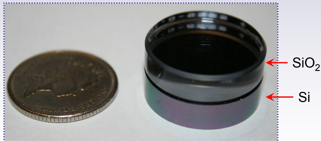
Silicon-silica hydroxy-catalysis bond
