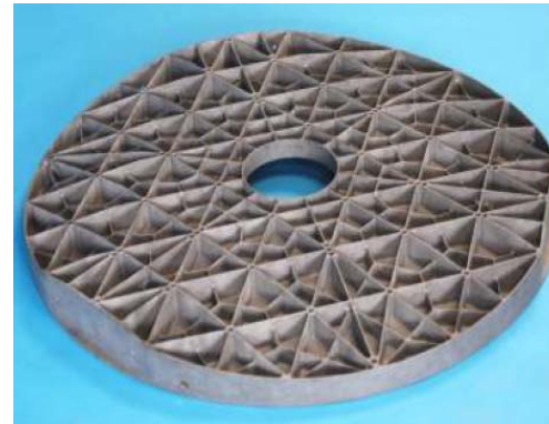
Si-C lightweighted telescope mirror (courtesy M. Krodel)
