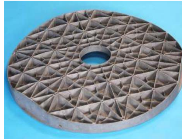
Si-C lightweighted telescope mirror (courtesy M. Krodel)
